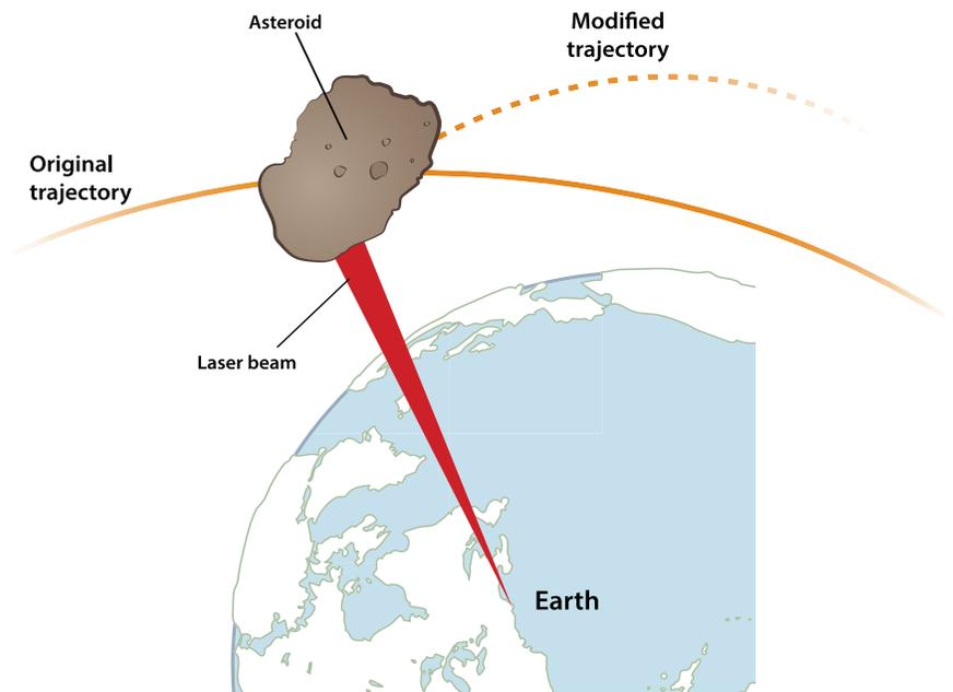
A high-intensity laser impacting with an object, such as space debris or a near-Earth asteroid, causes vaporization of surface material. This vaporization is called ablation, which produces thrust and can change the trajectory of the target object.
