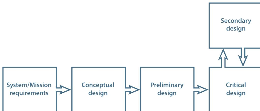
The process of designing aerospace technology begins with reviewing system and mission requirements. From this a conceptual design is developed. This phase is followed by the preliminary design phase in which concept designs are refined and preliminary parts are identified. The critical design phase follows and identifies finer details of the design. During this stage preliminary structure details are finalized and secondary structures are evaluated for inclusion in the critical design.
